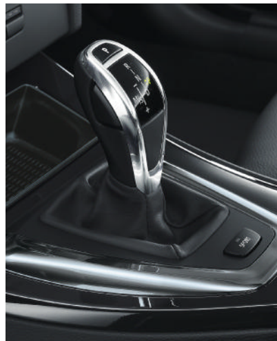
□ 7-speed sport automatic Double Clutch Transmission (DCT) provides smooth, lightning-quick gear changes and enhanced fuel efficiency by automatically shifting between two transmission structures. While one gear is disengaging, the next is already in position. Shift gears manually without a clutch by using steering wheel-mounted paddle shifters or the gear selector. (Available in 335is.)
