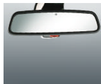
□ Automatic-dimming interior and exterior mirrors respond to the brightness of following headlights to minimize glare. A digital compass is integrated into the interior mirror. Both exterior mirrors are power-adjustable, with a fold-in function; the passenger-side mirror folds down to reveal the curb when in reverse gear.
