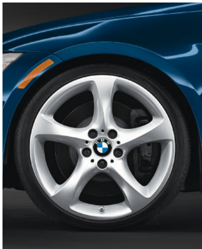
□ Star Spoke (Style 230) light alloy wheels with run-flat 1 performance tires 2 . In front: 19 x 8.0 wheels with 225/35 tires; in back: 19 x 9.0 wheels with 255/30 tires. 3 (Optional on 335i, requires Sport Package or M Sport Package.)
