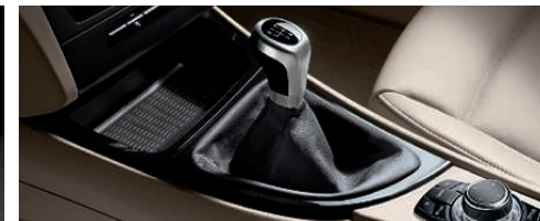
■ 6-speed manual transmission delivers a precise, athletic feel. Its responsiveness is due, in part, to the enhanced synchronization of shifts from neutral to each gear. A shortened shift lever and "throw" add to the sporty feel of the gearbox. The sixth gear drops revs at highway speeds for smooth cruising.
