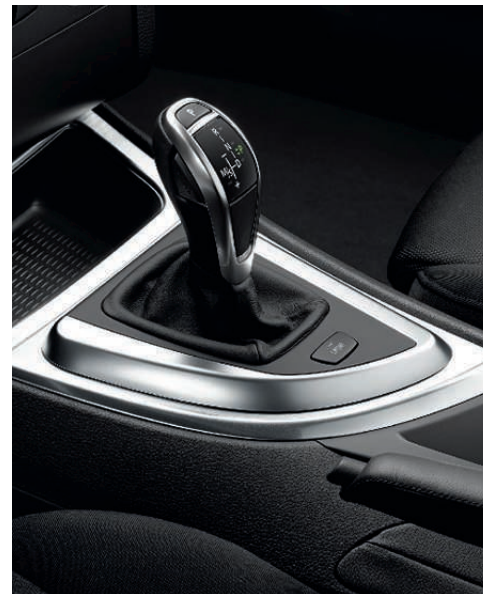
□ 7-speed Double Clutch Transmission (DCT) in the 135i achieves smooth, lightning-quick gear changes by automatically shifting between two transmission structures: while one gear is disengaging, the next is already in position. The result is quicker acceleration and enhanced fuel efficiency. You can also shift gears manually via steering wheel-mounted paddle shifters or by moving the gear selector lever forward/rearward.
