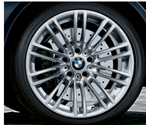
Double Spoke (Style 219M) Bright Silver finish light alloy wheels, 18 x 8.5 front, 18 x 9.5 rear; 245/40 front and 265/40 rear performance tires. 1
