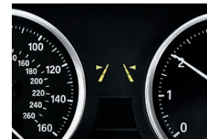
Lane Departure Warning feature alerts the driver by discreetly vibrating the steering wheel if the vehicle crosses lane markings without using the directional signal.
