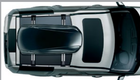
Luggage Box* VPLDR0062 Gloss Black Finish. Opens from both sides. Lockable for security. External dimensions: 69 inches/1,750mm long, 32 inches/820mm wide, 18 inches/450mm high. Volume 97 gallons/440 liters. Load capacity 165lbs/75kg † .
