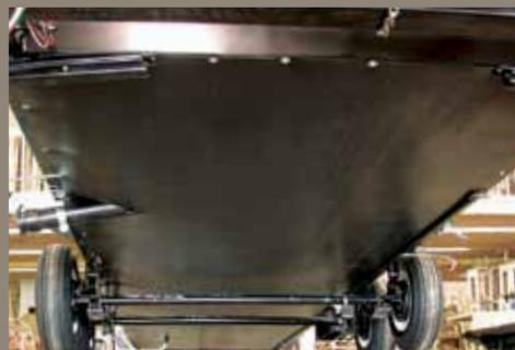
*The enclosed and underbelly eliminates turbulence caused by exposed frame members, holding tanks, plumbing etc.*
