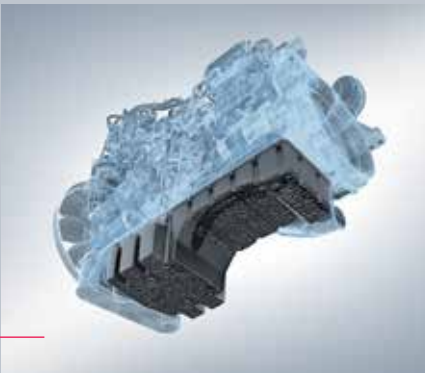
Plastic oil sump to save weight
