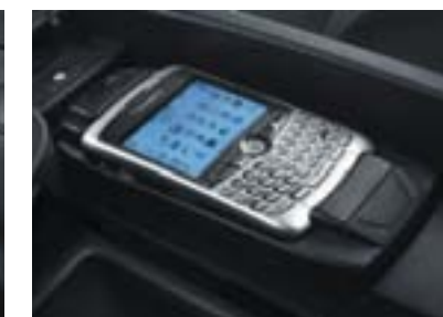
Snap-in adapter plays stored music, charges the phone and accesses the car antenna.
