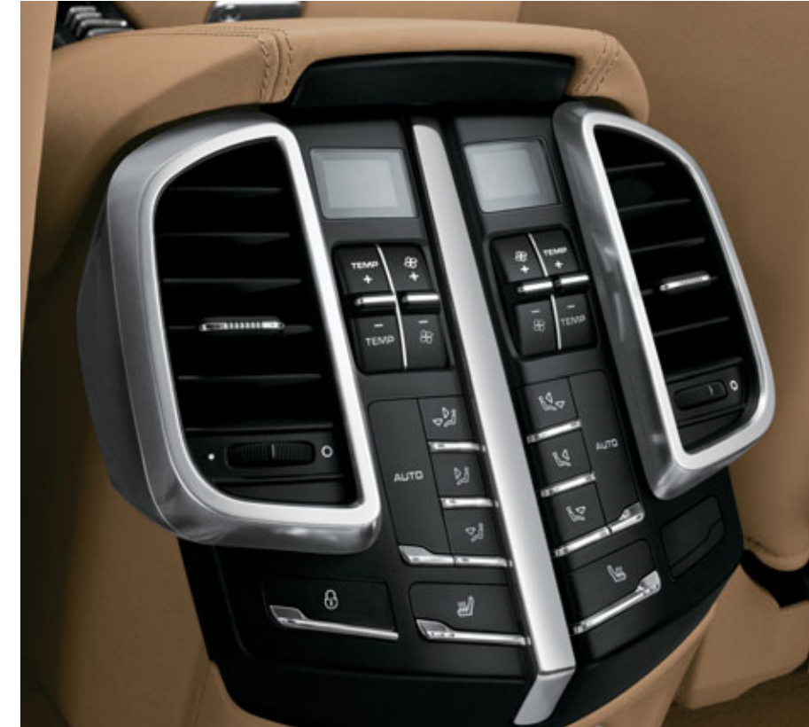
Four-zone climate control for rear seat area
