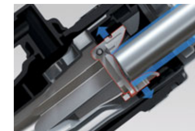
The blue outline shows the width of the diesel fuel nozzle, which is wider.
