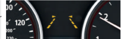
The Lane Departure Warning feature vibrates the steering wheel when your BMW crosses a line without first signaling.
