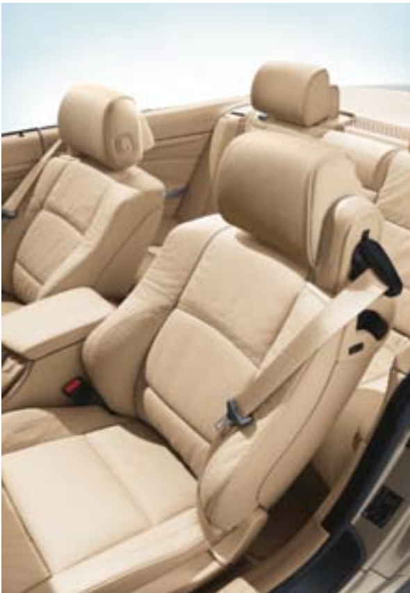
The three-point seat-integrated safety belt system offers excellent protection, with optimum belt geometry at all four seats.
