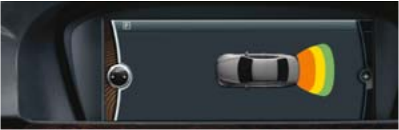
Park Distance Control uses ultrasonic sensors in the rear bumper to help you judge the distance to other cars and unseen objects when parking. The beeping becomes faster as your bumper approaches the object, turning into a constant tone when the distance is less than 12 inches.
