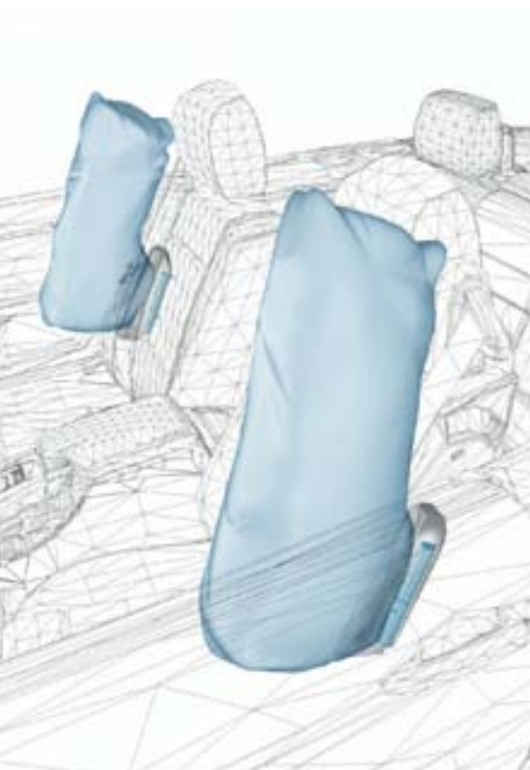
In a side impact, large seat-integrated side airbags are designed to provide head protection.
