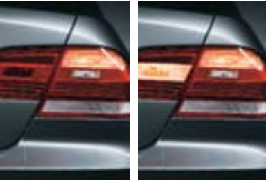
■ Adaptive Brake Lights help other drivers recognize the intensity of your braking actions. In emergency braking, the illuminated area of the brake lights increases, alerting drivers behind you to brake quickly.
