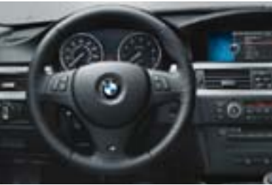
Three-spoke, leather-wrapped multi-function M sport steering wheel includes a thick, textured rim and thumb indents that are designed for performance driving, while multi-function buttons allow you to adjust various comfort features while keeping both hands on the wheel. The integrated multifunction buttons can be used to operate the radio, CD player and telephone (if installed).
