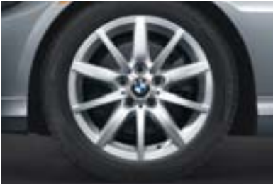
□ Star Spoke (Style 286) light alloy wheels and run-flat performance tires. 2 In front: 17 x 8.0 wheels and 225/45 tires; in back: 17 x 8.5 wheels and 255/40 tires. (Included in 328i Sport Package; optional in 328i xDrive, requires Sport Package.)
