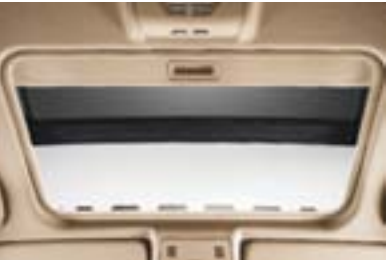
Two-way power glass moonroof with one-touch operation slides forward or tilts up to let in as much fresh air and sky as you like, while a wind deflector helps keep the wind out. Includes a sliding interior sunshade and remote operation.
