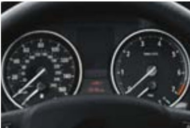
■ Instrument panel features a red backlit speedometer and tachometer. Centered between the two easy-to-read analog instruments is the on-board computer (at right) with liquid crystal display providing additional important driving information.
