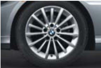
■/□ Multi Spoke (Style 284) 17 x 8.0 light alloy wheels with 225/45 run-flat¹ all-season tires . (Standard on 335i, 335i xDrive and 335d; included in 328i xDrive Sport Package.)
