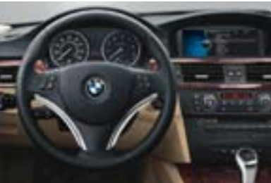
Three-spoke, leather-wrapped multi-function sport steering wheel lets you keep both hands on the wheel while adjusting various comfort functions, such as changing the radio, CD selections and volume. Voice command (included with Navigation system) can be used to change radio stations and audio selection, Navigation system destinations, and telephone entries.
