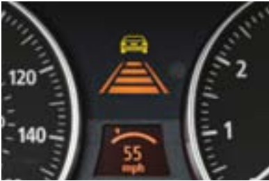
□ Active Cruise Control allows the driver to set a desired speed that is automatically maintained in free-flowing traffic. As a slower-moving vehicle is approached, a radar sensor alerts the system and adjusts speed to match the slower vehicle, while maintaining a preset following distance. As the lane ahead clears, the system automatically returns the car to the set speed. 2
