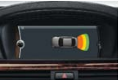
Park Distance Control uses ultrasonic sensors in the rear bumpers to help you judge the distance to other cars and unseen objects when parking. The beeping becomes faster as your bumper approaches the object, turning into a constant tone when the distance is less than 12 inches.
