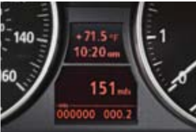
■ The on-board computer with Check Control provides feedback on the vehicle's operating status: oil level indicator and distance to next service appointment/oil change, as well as other detailed information, such as spark plug and micro-filter status. It also provides travel information, including travel range on remaining fuel, external temperature, and more.
