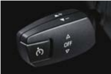
■ Dynamic Cruise Control lets you set and keep to a chosen speed above 20 mph, automatically applying the brakes downhill. It is activated via the left-hand steering column switch, and deactivated by applying the brakes or via the switch. 2
