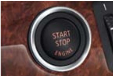
■ Engine Start/Stop button 1 and remote key control the engine. First, insert the remote key into the starter switch slot. After the electronic identification system confirms that it is the correct remote key, you can start (or later, turn off) the engine by pressing the Start/Stop button.
