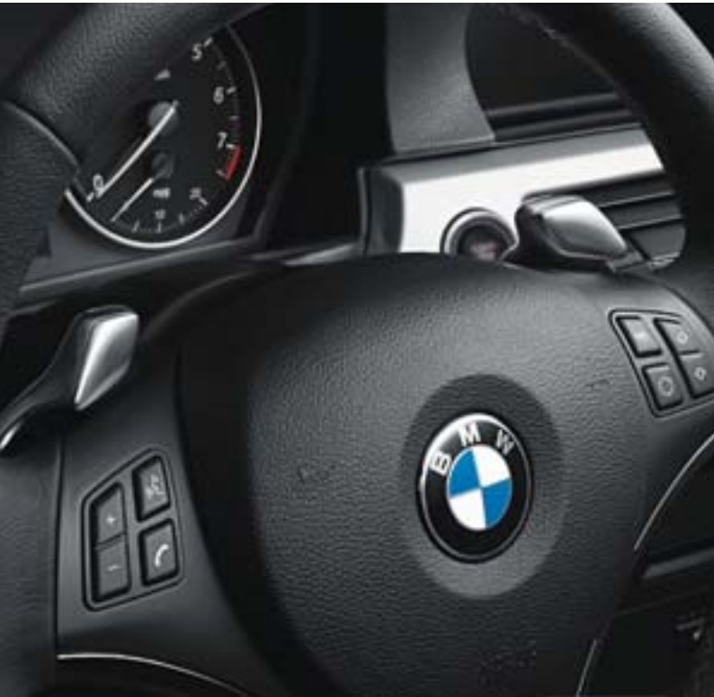
□ Three-spoke leather-wrapped multi-function sport steering wheel , with steering wheel-mounted paddle shifters that allow you to shift gears manually without using a clutch. This option is included in the 3 Series Sedan when equipped with the optional Sport Package and optional STEPTRONIC automatic transmission.
