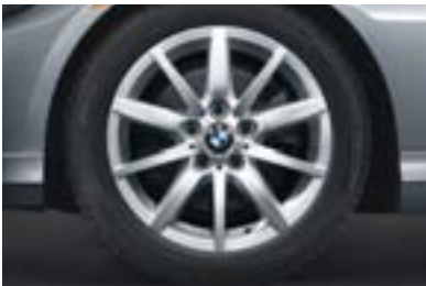
□ Star Spoke (Style 286) light alloy wheels and run-flat¹ performance tires.² In front: 17 x 8.0 wheels and 225/45 tires; in back: 17 x 8.5 wheels and 255/40 tires. (Included in 328i Sport Package; optional in 328i xDrive, requires optional Sport Package.)
