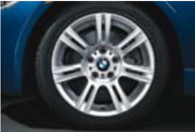
Double Spoke (Style 194M) M light alloy wheels and run-flat performance tires. 2 In front: 17 x 8.0 wheels and 225/45 tires; in back: 17 x 8.5 wheels and 255/40 tires. (Included in 328i and 328i xDrive M Sport Package.)
