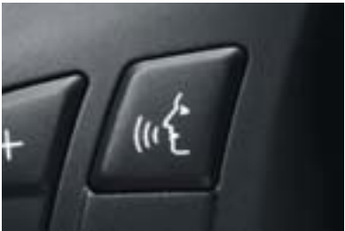
□ Voice Activation allows you to activate numerous Navigation system functions, record up to five minutes of notes, and dial hands-free. The Voice Activation button must be pressed before each use, so conversations won't accidentally activate the phone or other systems.
