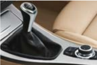
■ 6-speed manual transmission delivers a precise, athletic feel. Its responsiveness is due, in part, to the enhanced synchronization of shifts from neutral to each gear. A shortened shift lever and "throw" add to the sporty feel of the gearbox. The sixth gear drops revs at highway speeds for smooth cruising. (Shown with iDrive, included with optional Navigation system.)
