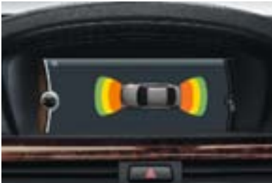
□ Park Distance Control uses ultrasonic sensors in the front and rear bumpers to help you judge the distance to other cars and unseen objects when parking. The beeping becomes faster as your bumper approaches the object, turning into a constant tone when the distance is less than 12 inches.
