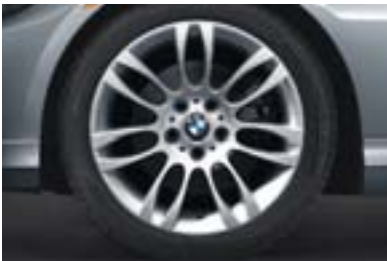
□ Double Spoke (Style 195) light alloy wheels and run-flat¹ performance tires.² In front: 18 x 8.0 wheels and 225/40 tires; in back: 18 x 8.5 wheels and 255/35 tires. (Included in 335d Sport Package.)
