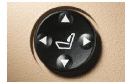
Lumbar support for front seats adds four-way adjustable comfort for the lower back. Lumbar support can be adjusted up/down and in/out.
