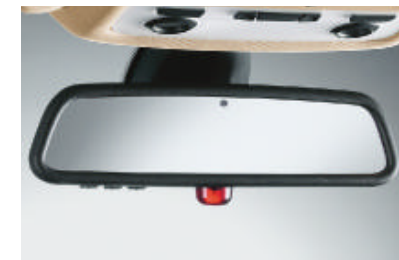
The automatic-dimming inside rear-view mirror darkens in response to the bright headlights of vehicles behind you. The easy-to-read digital compass , integrated into the mirror, is a convenient way to constantly keep your bearings while driving.
