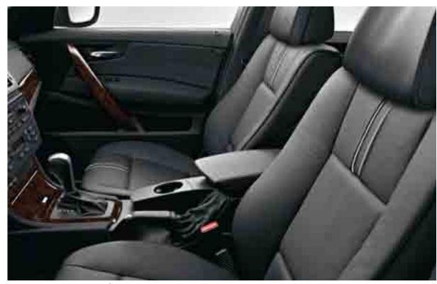
□ **16-way power Comfort seats**¹ for the driver and front passenger provide optimum lateral support during tight cornering thanks to specially padded, highly contoured side bolsters while remaining exceptionally comfortable when driving over long distances. The seats have individual power adjustment for seat height, backrest angle, seat bottom angle, forward/backward position, and thigh support.
