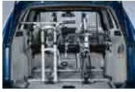
Floor cargo rails are designed for use with accessory storage racks for clean, safe stowage of items in the cargo area. Luggage compartment bike rails (sold separately as a BMW accessory) secure the frames after removing the front wheels. NOTE: Bicycles shown are not sold with the X3 SAV.®
