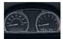
■ Instrument panel has analog display for speedometer and tachometer with integrated fuel and engine temperature gauges. Also includes an LCD display for mileage, trip odometer, and on-board computer (if so equipped). When parking lights or headlights are on, the gauges are in an easy-to-read red.
