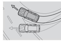
■ Dynamic Stability Control (DSC) provides remarkable tenacity on slippery road surfaces. If the system senses over- or understeer, it modulates engine power and can apply brakes individually to help keep the vehicle under control and going in the intended direction.
