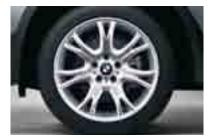
☐ **Y Spoke (Style 191M)** 19 x 8.5 front, 19 x 9.0 rear light alloy wheels and 235/45 front and 255/40 rear performance tires<sup>1</sup> are available as an option when ordering the Sport Package.
