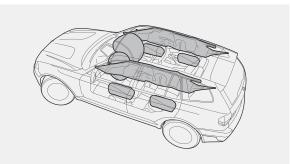
The X3 offers a full complement of airbags, front and rear. BMW s HPS (Head Protection System) helps cushion and protect the heads of occupants seated by the doors.
