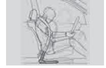
■ In the event of a severe frontal collision, automatic safety-belt pretensioners automatically tighten the lap and shoulder belts around front-seat occupants. Always wear your safety belt and always place children in the rear seat.
