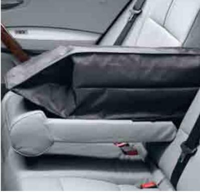
Cargo bag allows for clean transport of up to four pairs of skis with up to four occupants in the car; whenever the cargo bag is not in use, it remains stored conveniently and out of sight behind the rear center armrest. (Upon BMW X3 SAV® delivery, the cargo bag shown is detached and stored beneath the load floor in the rear cargo area.)
