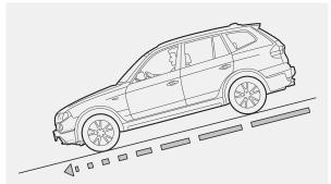
Hill Descent Control (HDC) lets the BMW X3 tackle steep downhill slopes with ease, while it helps stabilize the X3 s handling. When you engage HDC, it automatically applies the brakes and slows the engine, keeping your speed constant without riding the brakes.
