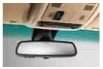
The automatic-dimming inside rear-view mirror darkens in response to the bright headlights of vehicles behind you. The easy-to-read digital compass, integrated into the mirror, is a convenient way to constantly keep your bearings while driving, and upon arriving home, the BMW Universal garage-door opener offers convenient remote functions, such as opening garage doors or turning on household lights.
