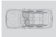
■ In the event of a collision, only the airbags that are needed are deployed. For the driver and front passenger, this includes front airbags, door-mounted side-impact airbags, and Head Protection System (HPS). For rear-seat passengers this includes HPS and optional rear side-impact airbags.
