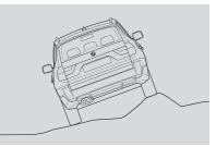
■ The roll-over sensor is networked with the Dynamic Stability Control system to enable critical situations to be identified faster and more effectively. If the vehicle threatens to overturn, airbags and safety-belt pretensioners are deployed immediately for maximum passive safety.
