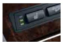
Heated front seats are a welcome feature in cooler weather. With the touch of a button, driver and front passenger can individually select from three heat settings.
