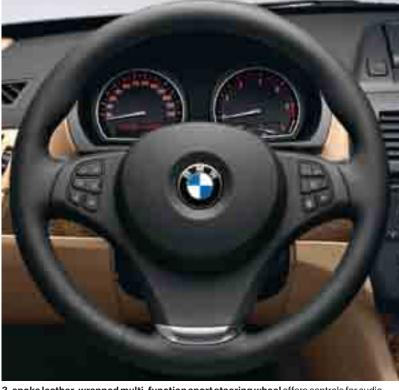
**3-spoke leather-wrapped multi-function sport steering wheel** offers controls for audio system, cruise control and (accessory) phone.
