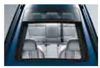
Dual-glass-panel **Panoramic moonroof** features fully electric slide and lift control. Includes trap release, comfort opening/closing function, a wind deflector to help keep the wind out, and an electric sun shade to help shield cabin from excessive heat.
