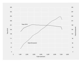
Torque-rich, free-revving and uncommonly smooth: the X3 s inline six eagerly revs to 7000 rpm, producing 260 horsepower at 6600 rpm and 225 lb-ft of torque at just 2750 rpm.
