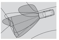
☐ Xenon Adaptive Headlights with Corona headlight-rings automatically swivel to follow the curves of the road. The system uses data from on-board sensors and the steering wheel angle to determine the car s direction, then adjusts the headlights accordingly, for excellent nighttime vision.
