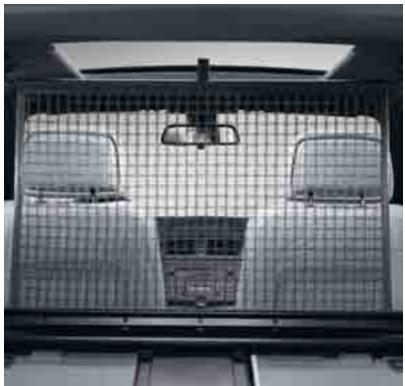
☐ Retractable cargo net helps keep pets and cargo securely away from the passenger area. Net can be anchored behind the back seats; when both back seats are folded, it can be anchored behind the front seats. When not in use, the luggage net housing can easily be removed.
