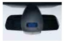
■ Rain sensor uses infrared light to measure the amount of rain. When the wipers are in the intermittent mode, the rain sensor automatically adjusts the windshield-wiping interval as needed. Automatic headlight control (not shown), included with rain sensor, activates headlights by means of a sensor that responds to darkness.
