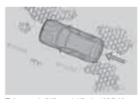
■ Automatic Differential Brake (ADB-X) is similar to the function of a differential lock, braking each wheel independently, as needed. As soon as wheelspin is detected at any wheel, ADB-X applies that brake automatically until the wheel regains traction. DSC assists ADB-X by modulating the amount of power sent to each wheel; with DSC turned off, full power continually flows to all four wheels.
