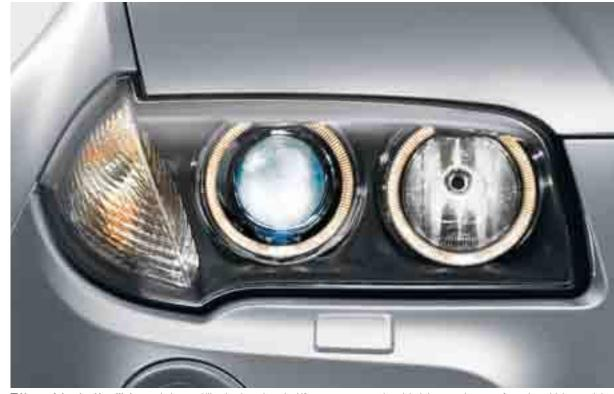
□ Xenon Adaptive Headlights optimize road illumination when the X3 enters a curve or bend, helping to enhance safety when driving at night. Sensors continuously monitor the angle of the steering wheel, the vehicle s speed, yaw and other factors to determine the direction in which the X3 is heading. The headlights swivel accordingly, up to 15 degrees left or right.
