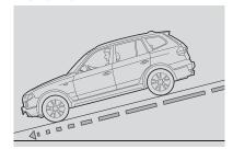
■ Hill Descent Control (HDC) helps the X3 drive down steep hills without having to ride the brake. By pressing the HDC button, the system keeps the X3 s speed under control automatically.
