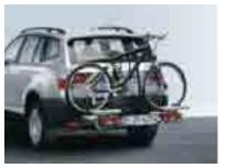
Rear-Mounted Bicycle Carrier carries two locked bicycles; an extension set holds a third. Even when in use, tailgate can be opened.
