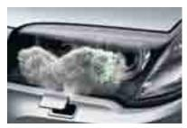
High-intensity retractable headlight washers help keep lights clean of ice, mud, road salt and other coatings, for maximum road lighting and enhanced driving visibility.
