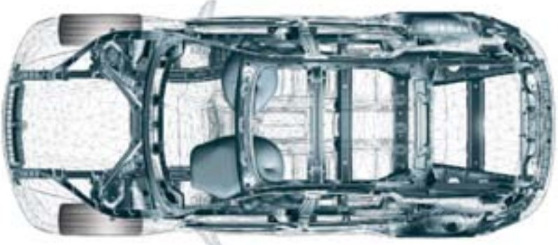
In the event of a severe impact, the X6's extremely rigid steel structure is designed to route impact forces around the passenger cell, and deform in a predetermined way. The BMW Advanced Safety System coordinates the activation of airbags, head restraints, safety-belt pretensioners and more, all helping to protect you and your passengers.
